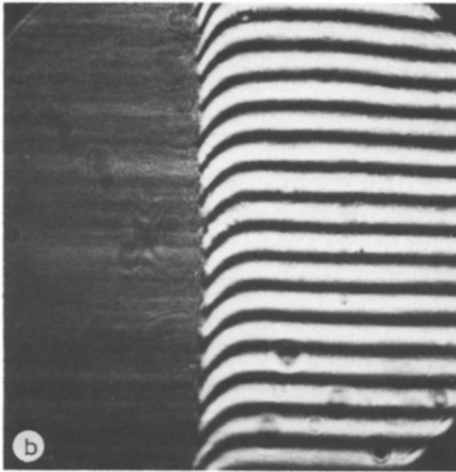
Fig. 3. Interferograms of 5% saccharose aqueous solution near a 0.2-mm layer of silica gel (DC-Plastick-folien Kieselgel 60, Merck) after 10 (a), 60 (b) and 180 sec (c).
